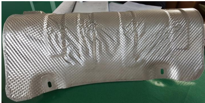
Fig. 3 Heat protector parts of aluminum alloy sheet
