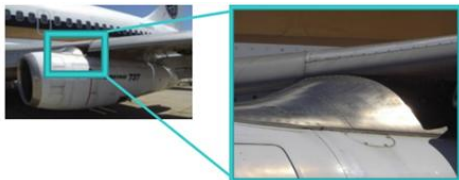
Fig 1. Countersunk rivets on the engine pylon of a Boeing 737 aircraft
