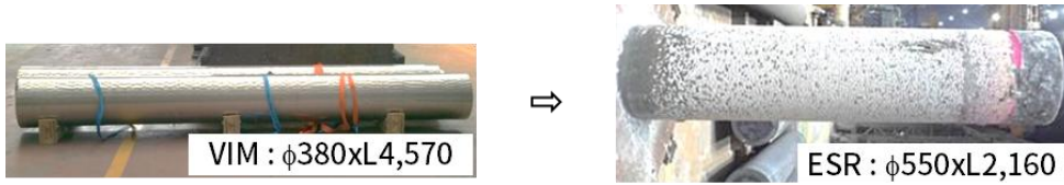
Fig. 1 Photograph of manufactured ingots by using the VIM+ESR process
