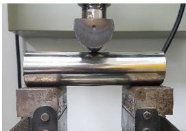
Fig. 3 Lateral three-point tube bending test
