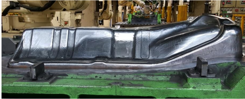
Fig. 2 Heat protector die for drawing aluminum alloy sheet
