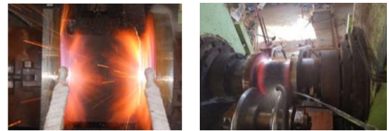
Fig. 6 Forming test of coupling
