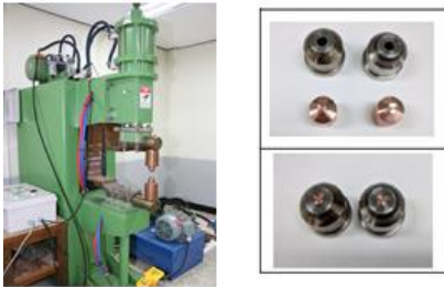
Fig. 2 Electric resistance spot welding machine using heated dies and copper electrode
